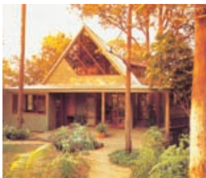
Stained, preservative treated, grooved plywood cladding blends with bushland setting
